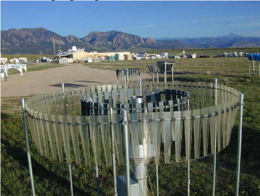
Figure 6.b Double Alter (Rain Gauge) Wind Shield surrounding a Geonor Weighing Gauge (automated)
