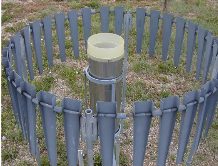
Figure 6.a Alter (Rain Gauge) Wind Shield surrounding an 8 inch Standard Rain Gauge (manual)
